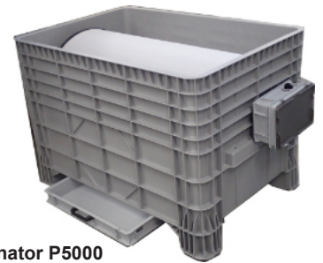
Pollinator P5000 Capacity: ~5000 g Screen: 150 micron
